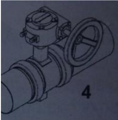
Connection of valve and piping with gasket
